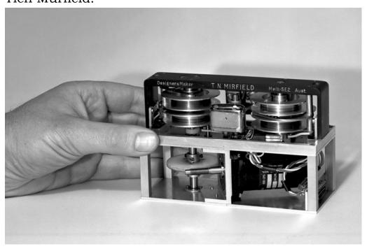
And this photo shows David with the first flight recorder in a box that would survive a crash. It is held today at the DSTO laboratory in Melbourne where it was invented.
