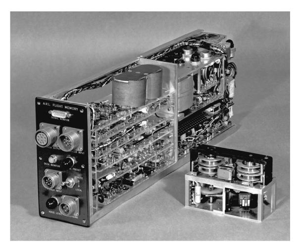
This photo compares the pre-production model with the original experimental one on the right.....you can see the level of sophistication and complexity has increased by an order of magnitude.
